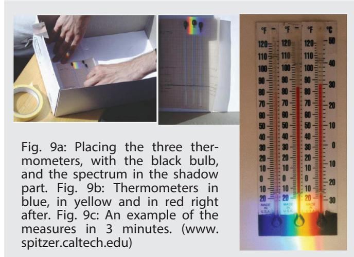
Fig. 9a: Placing the three thermometers, with the black bulb, and the spectrum in the shadow part. Fig. 9b: Thermometers in blue, in yellow and in red right after. Fig. 9c: An example of the measures in 3 minutes. (www.spitzer.caltech.edu)
