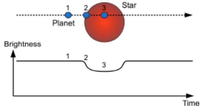
Fig. 20b: The transit method for planet detection
