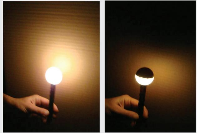
Fig. 16a: Lamp without shield. Fig. 16b: Shielded Lamp.
