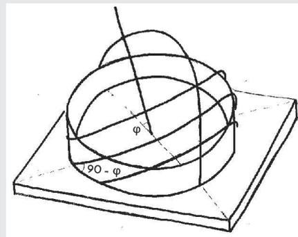
Fig. 12: Model showing the horizon and polar axis.
