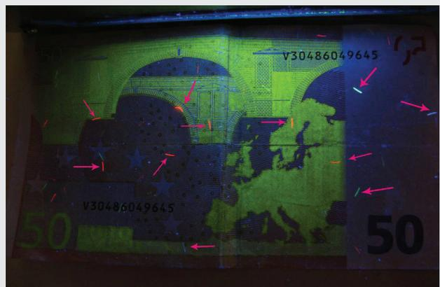
Fig. 18: A note of 50 € illuminated with UV light, shows small fluorescent strips marked here by arrows.
