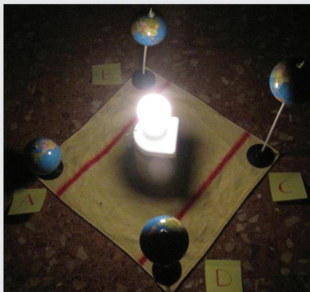
Fig. 3: Model of the revolution motion that explains seasons. When the Earth is at position A it is summer in the northern hemisphere and winter in the southern hemisphere. When the Earth is at position C it is winter in the northern hemisphere and summer in the southern hemisphere. And when the Earth is at positions B and D hemispheres are equally illuminated and equinoxes take place. Then, daytime and nighttime are equal.
