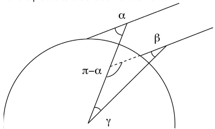
Fig. 19: Placement of plumbs and angles in the Eratosthenes experiment.
