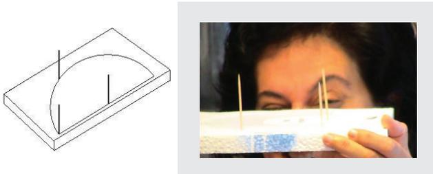
Fig. 7a and 7b: Using the horizontal goniometer.
