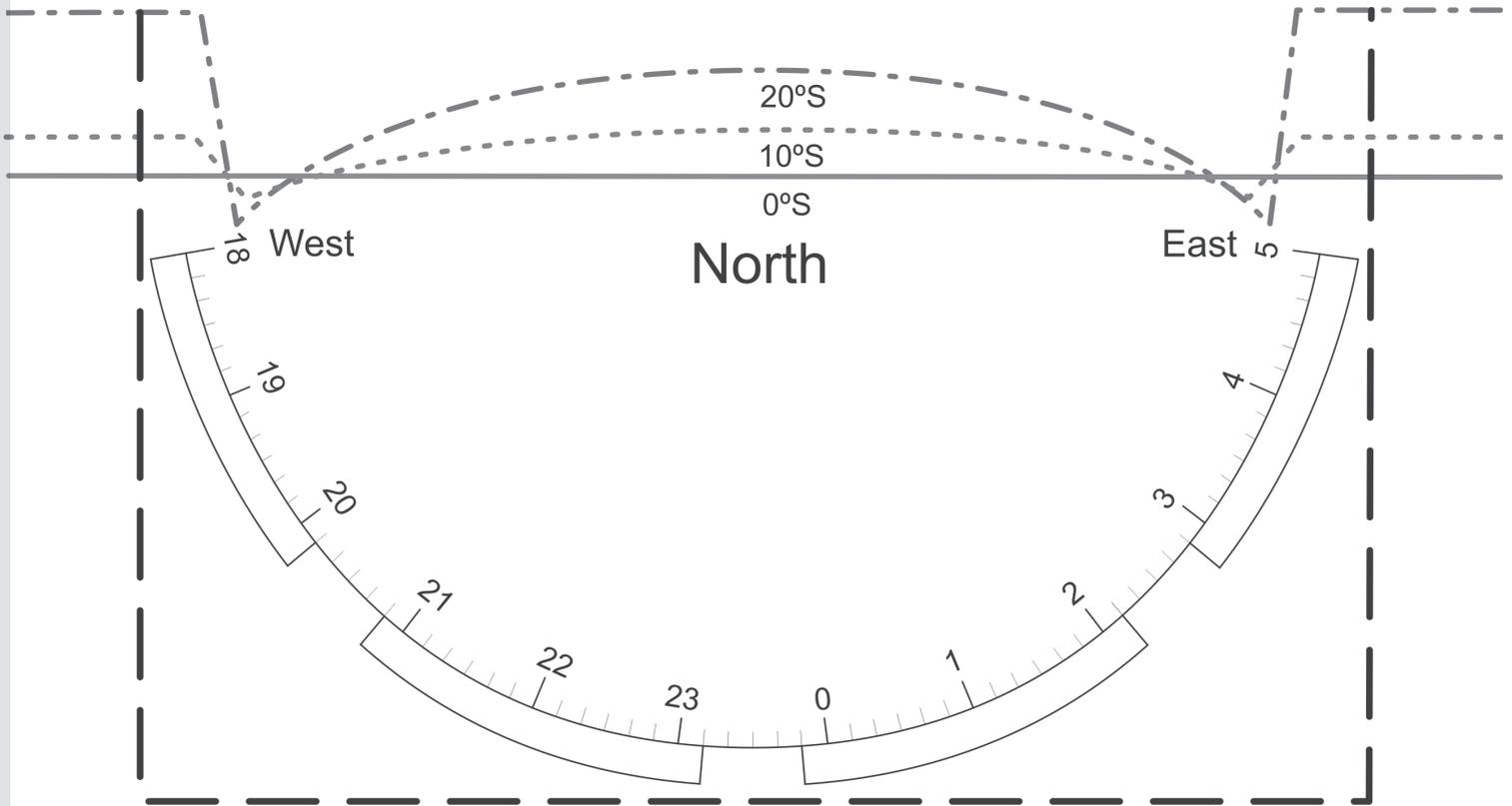
Fig. 9b: Pocket for the southern horizon in northern hemisphere (latitude 0, 10 and 20 North).
