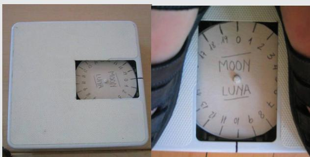
Fig. 13a and 13b: Bathroom scale with the replaced disk.
