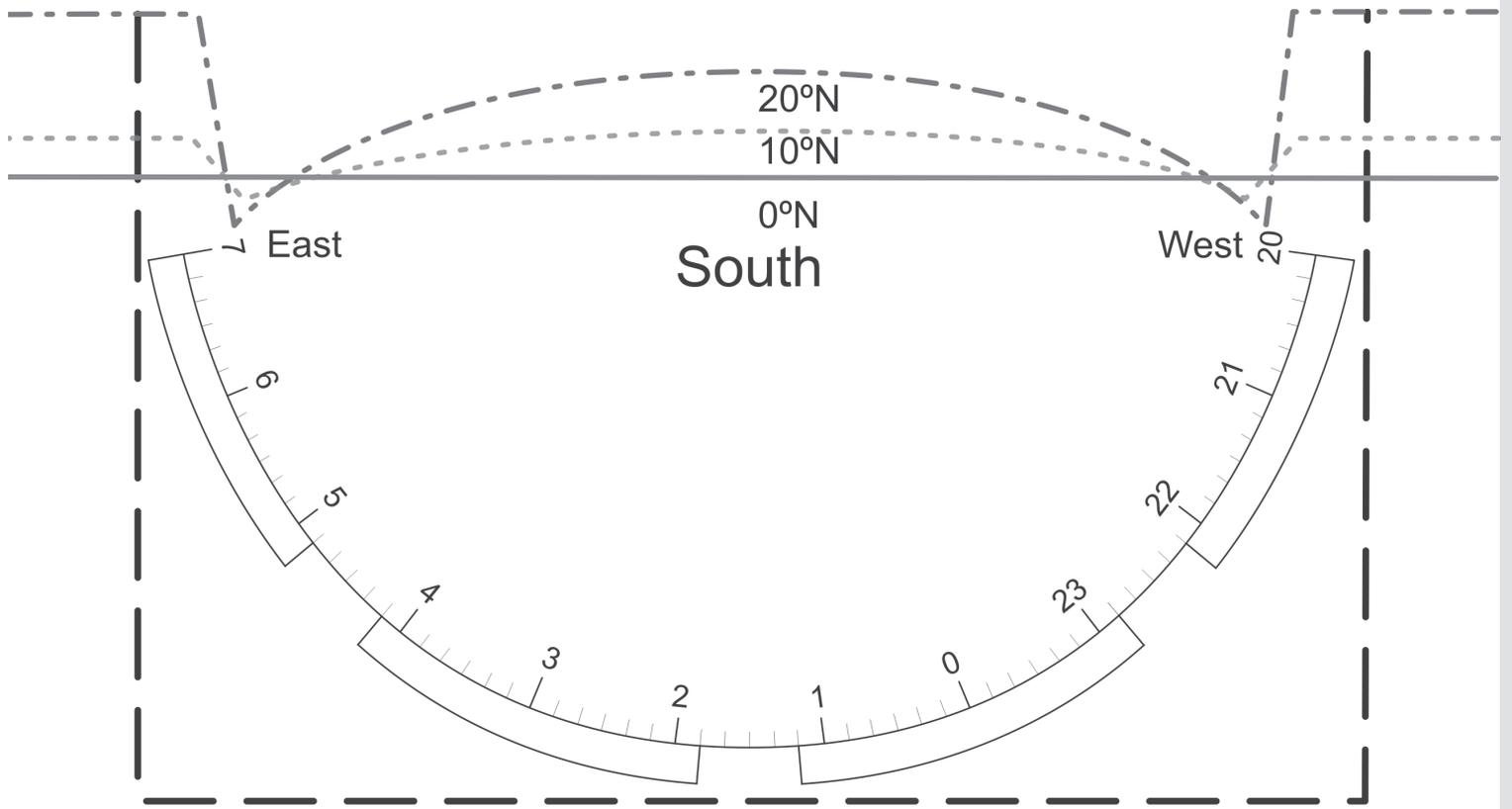
Fig. 9b: Pocket for the northern horizon in southern hemisphere (latitude 0, 10 and 20 South).
