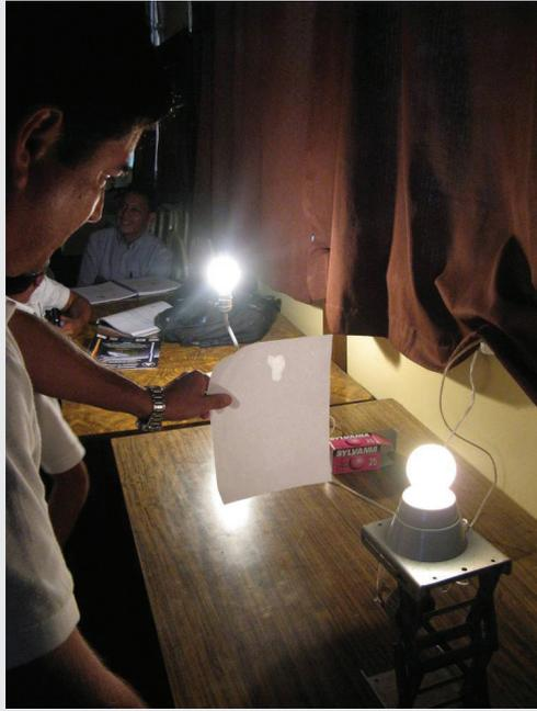
Fig. 16: Oil slick photometer, between two light bulbs.
