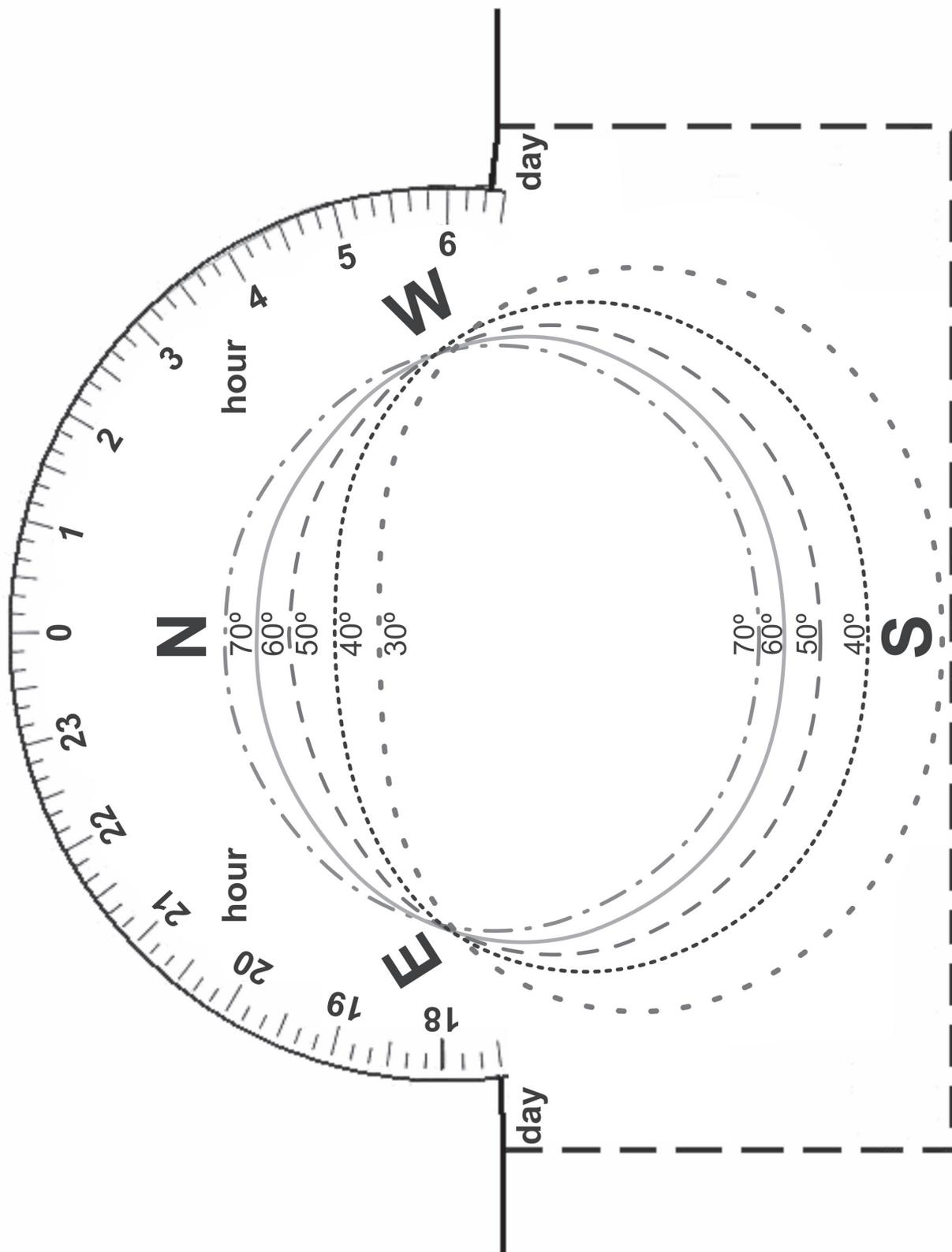
Fig. 9e: Pocket for both horizons in northern hemisphere. Latitudes 30, 40, 50, 60 and 70 North.
