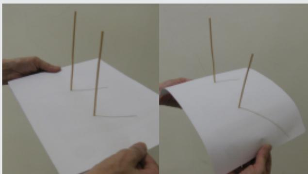
Fig. 18a and 18b: In the flat surface the two sticks produce the same shadow, but when the surface is curved shadows are different.
