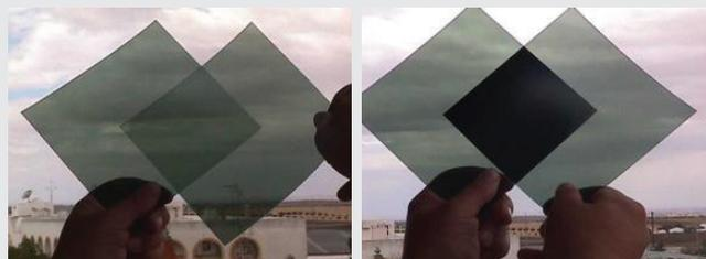
Fig. 4a: If the filters have the same orientation, light passes through.
