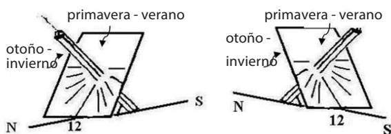
Fig. 23: Equatorial clock used in northern hemisphere.
