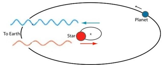
Fig. 20a: The radial velocity (RV) method for planet detection
