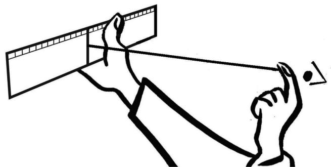
Fig. 2: Using the instrument (a ruler and a piece of string 57 cm long), we can measure angles with the equivalence "1cm = 1°".
