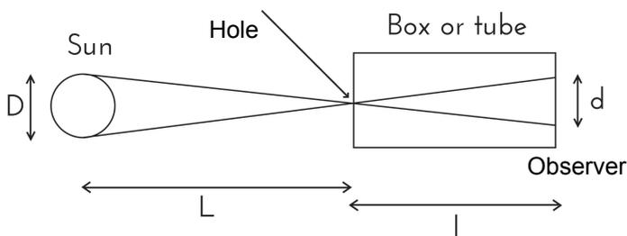
Fig. 14: Underlying geometry of calculation.
