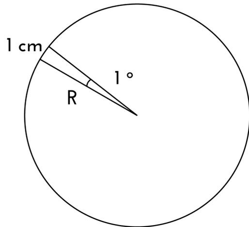
Fig. 1: The radius R in order to obtain an instrument where 1° is equivalent to 1 cm.
