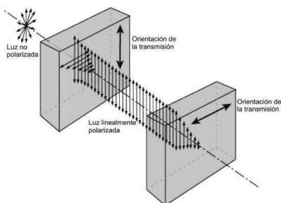
Fig. 3: When two filters have a perpendicular transmission orientation, the light which passes through the first is blocked by the second.
