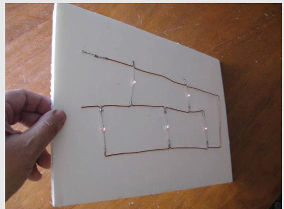
Fig. 13a and 13b: Cassiopeia made with infrared leds. They are connected in parallel.
