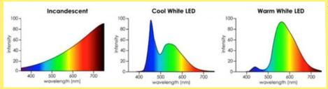
Attached is the spectrum of light from an LED bulb and a filament bulb.
