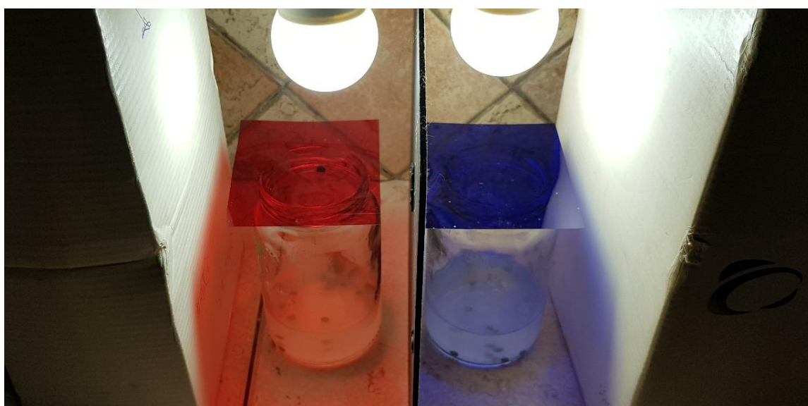
Fig. 17 and 18: The solution and the lamps with red filter and with blue filter.
