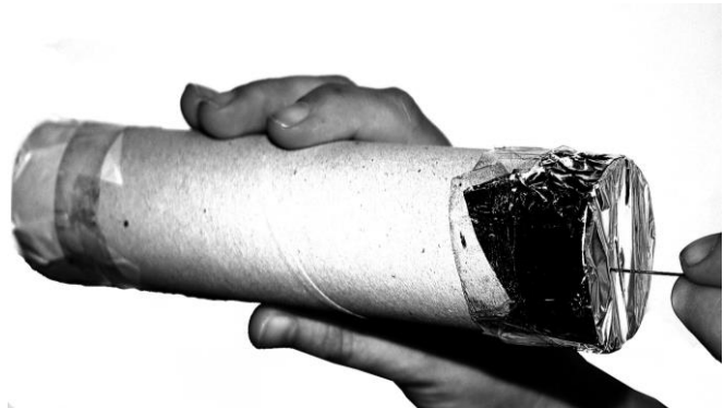
Fig. 12 and 13: Model of the pinhole camera.
