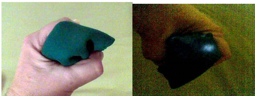
Fig. 12a and 12b: Felt completely blocks visible light but not infrared.
