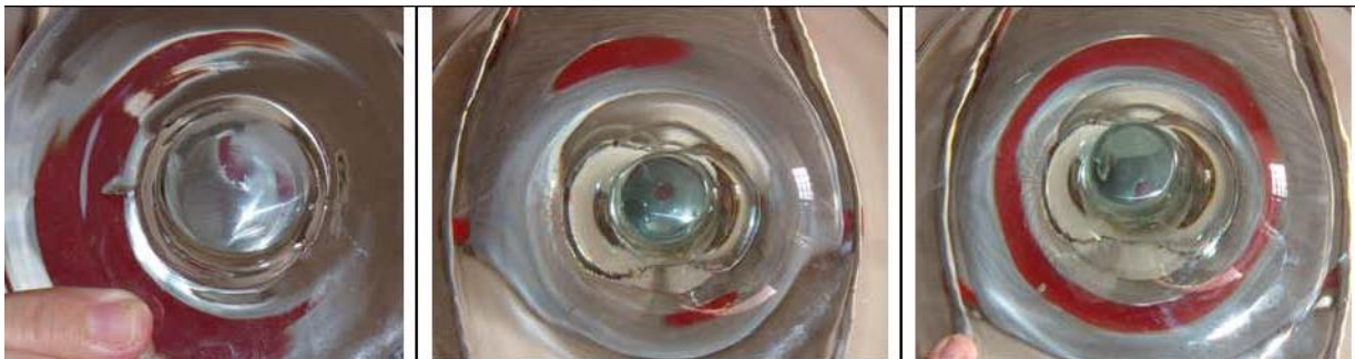
Fig. 24a, Fig. 24b and Fig. 24c: The glass foot can simulate various shapes made by gravitational lenses: arc segments, images of points, and Einstein rings.
