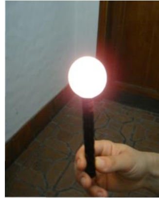
Fig. 15b: Flashlight with the tennis table ball simulating the street lamp
