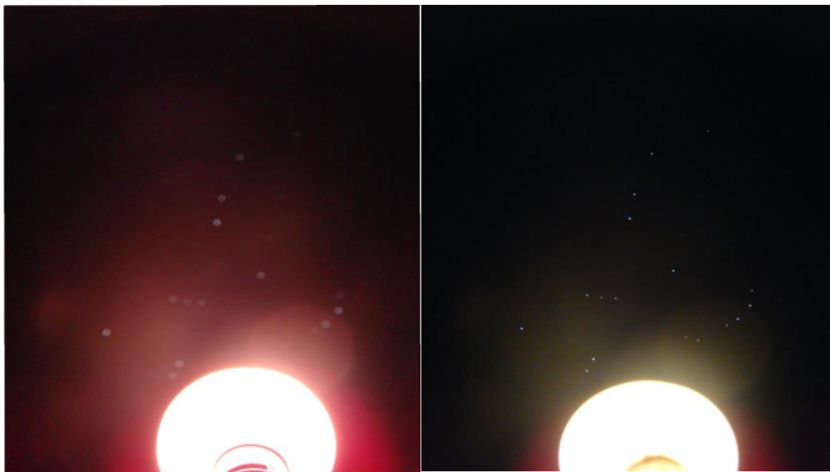
Fig. 17a: Appearance of the night sky with lanterns without shielded. Fig. 17b: Appearance of the night sky with lights shielded
