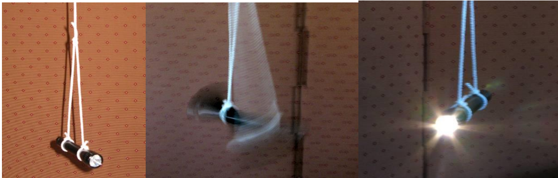
Fig. 17a: Assembly, Fig. 17b: Spinning the flashlight, Fig.17c: As it spins we observe the beam of light in a periodic way
