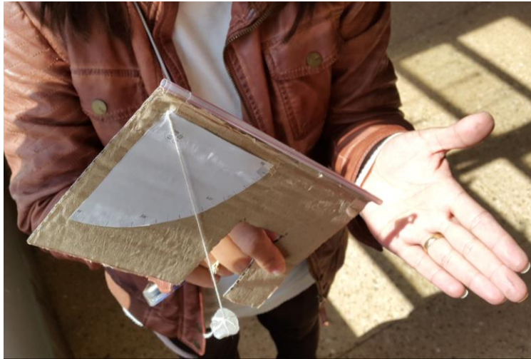
Figure 12. Use of the quadrant by projection.
