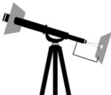
Fig. 10a: Solar observation by projection with a telescope (never look directly at the Sun).
