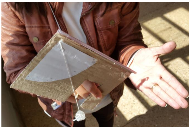
Figure 12. Use of the quadrant by projection.
