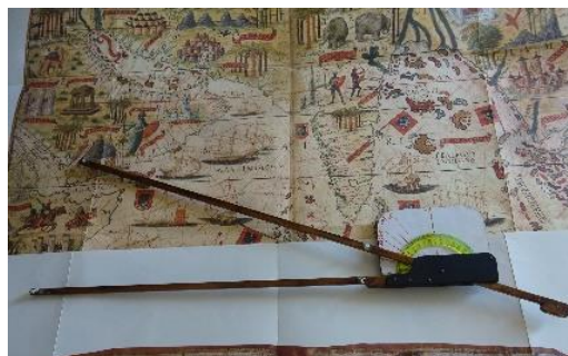
Fig.17: Karmal Very simple instrument for determining latitude. Own source
