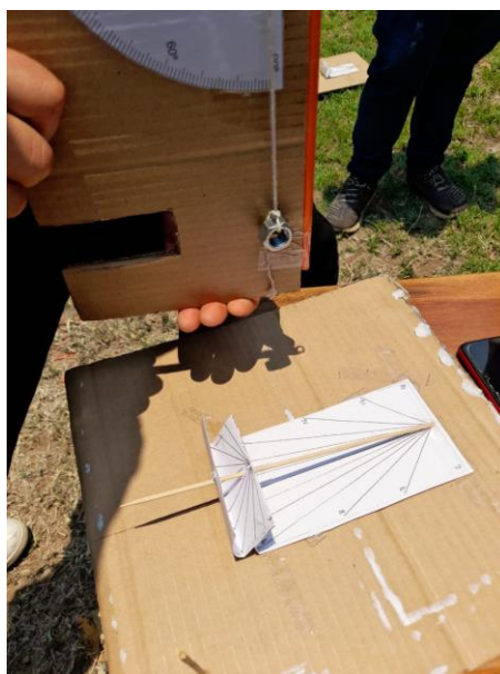
Fig 2: Measurement of the altitude of the Sun during the passage of the Sun through the zenith. It was found that the altitude of the passage through the zenith at solar noon was 90^\circ .
