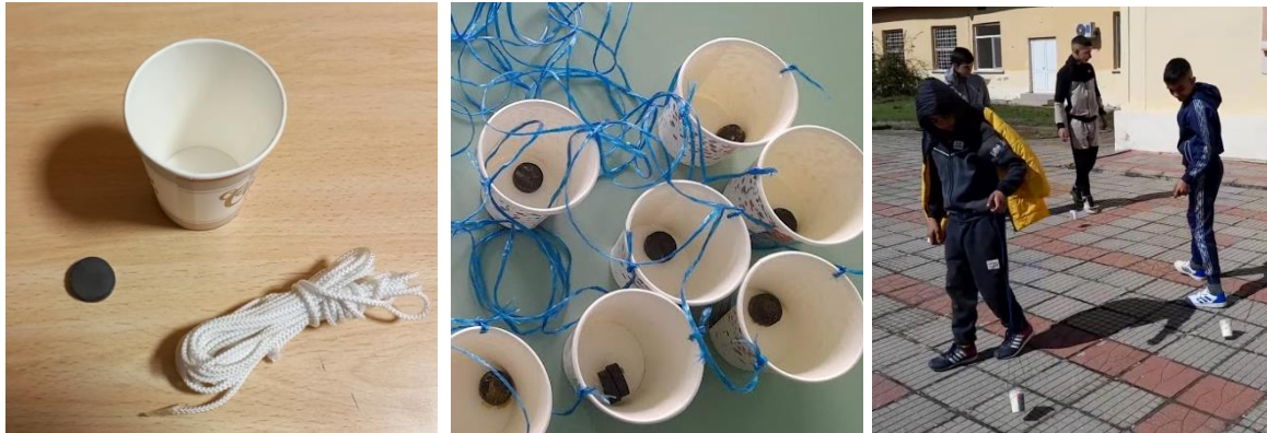
Fig. 29a and 29b: The glass tied with a thread and a small magnet inside. Fig. 29c: Student using the beaker, searching for micrometeorites.
