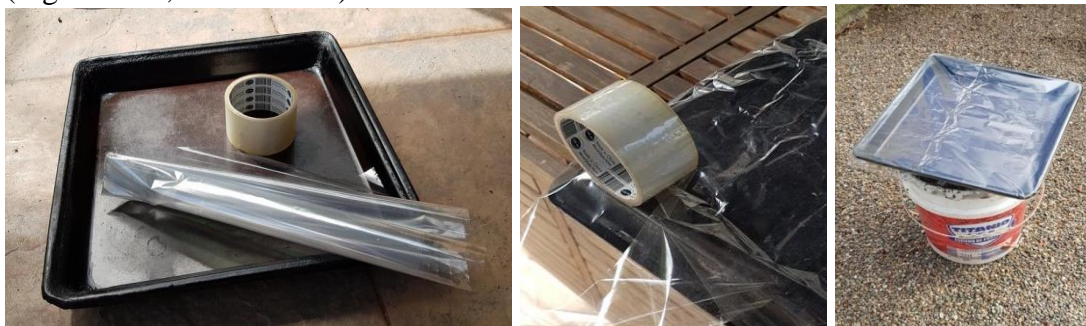
Fig. 28a: Tray, cellophane and tape, Fig. 28b: Gluing the cellophane to the back of the tray, Fig. 28c: Micrometeorite “trap” set up in the garden.
