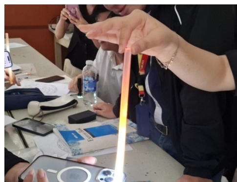
Fig. 18. The white light from the flashlight scatters as it passes through the stick, just like sunlight in the atmosphere.
