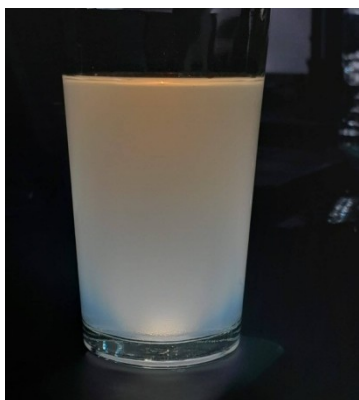
Fig. 15 The light from the flashlight that comes out from the side of the glass appears bluish.
