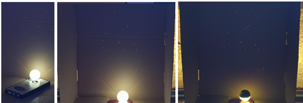
Fig. 16a, 16b and 16c: Experience using the luminaire (ping pong ball with and without shielding, on the LED light of the mobile phone).
