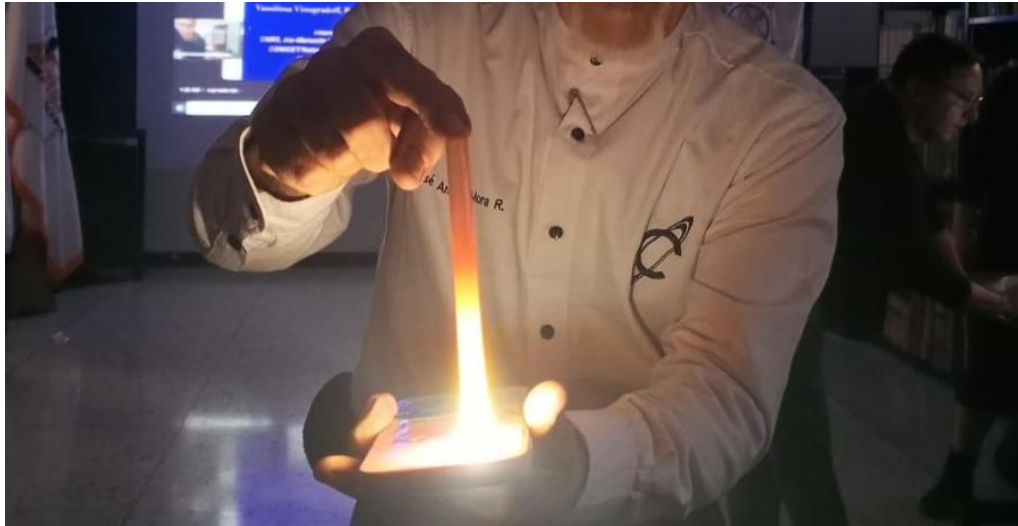
Fig. 25: The hot-melt silicone stick near the mobile phone's light appears bluish, but in the area furthest from the light it appears yellowish and reddish.
