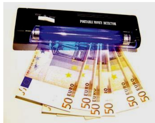
Fig. 18b: Counterfeit Detector, which uses ultraviolet light
