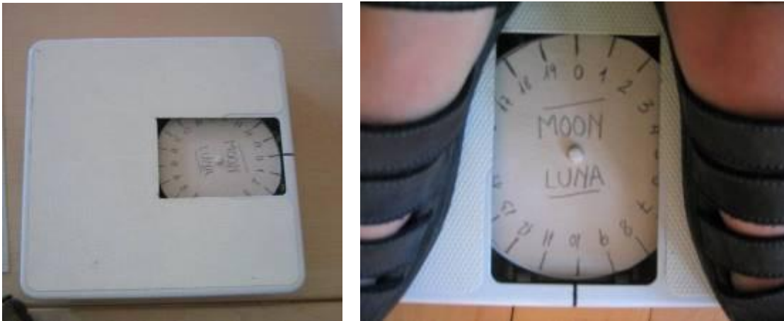
Fig.13a and 13b: Bathroom scale with the replaced disk.
