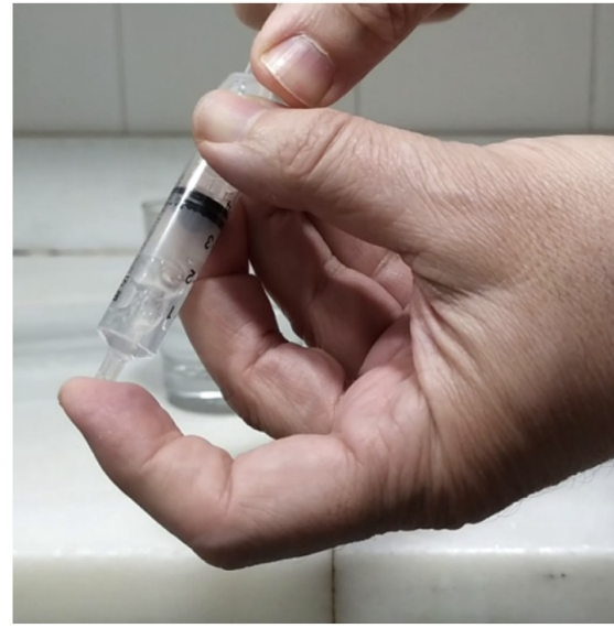
Reducing the interior pressure would cause water to boil even below 100 C.
