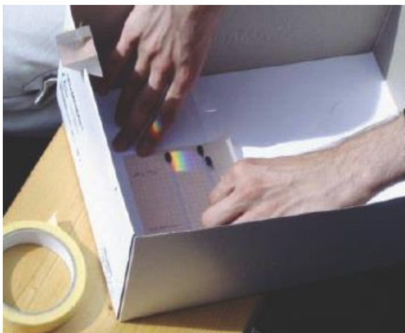
Fig.10a: Placing the three thermometers, with the black bulb, and the spectrum in the shadow part.
