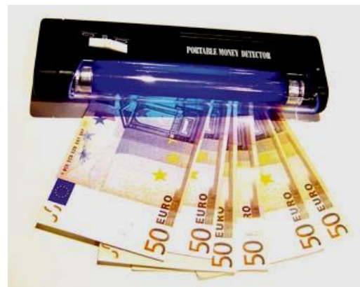
Fig. 18b: Counterfeit Detector, which uses ultraviolet light
