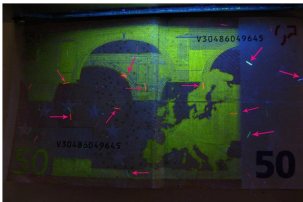
Fig. 18a: A note of 50 € illuminated with UV light, shows small fluorescent strips marked here by arrows.
